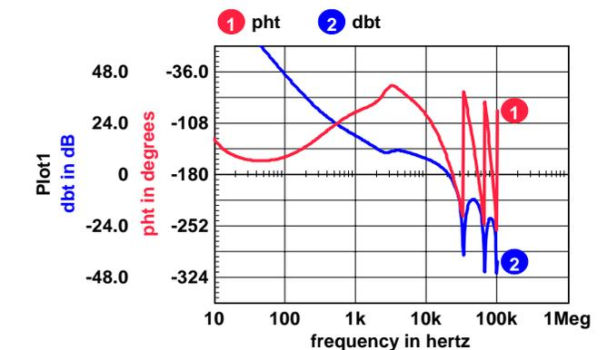
Figure 8: The GFT used with the Average model shows small phase margin between 10 and 100Hz
