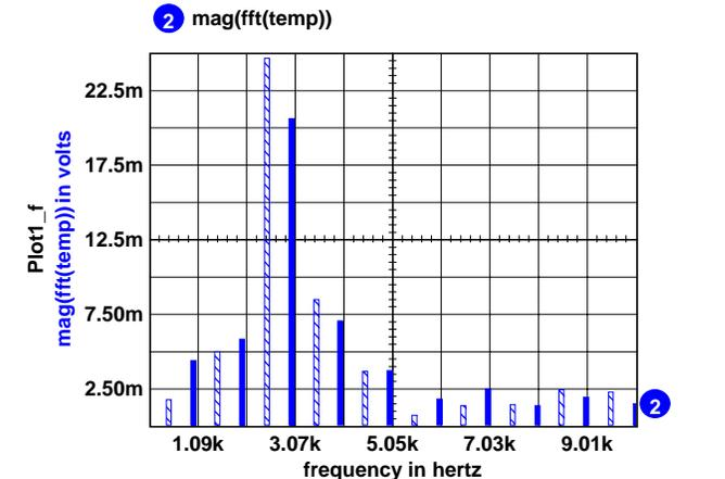
Figure 6: Power Spectral Density shows noise spread about the average switching frequency.
